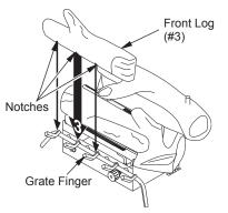
Figure 31 - Installing Front Log (#3) (Base may very from illustration)
